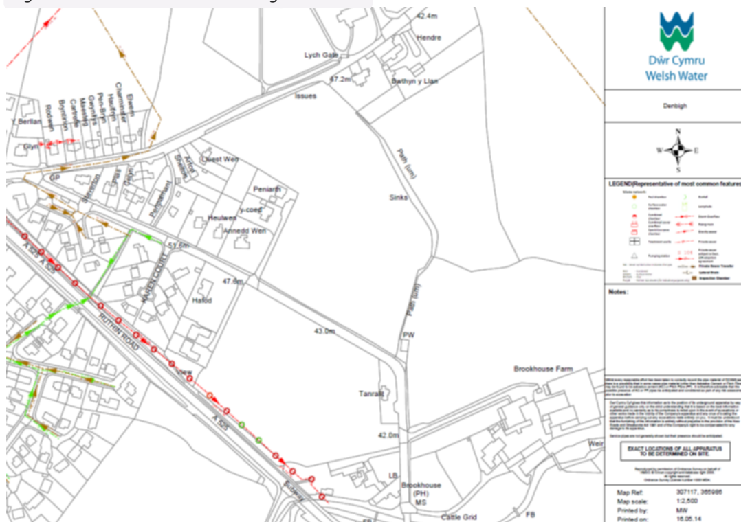
Figure 10 : Local water and sewerage network.
